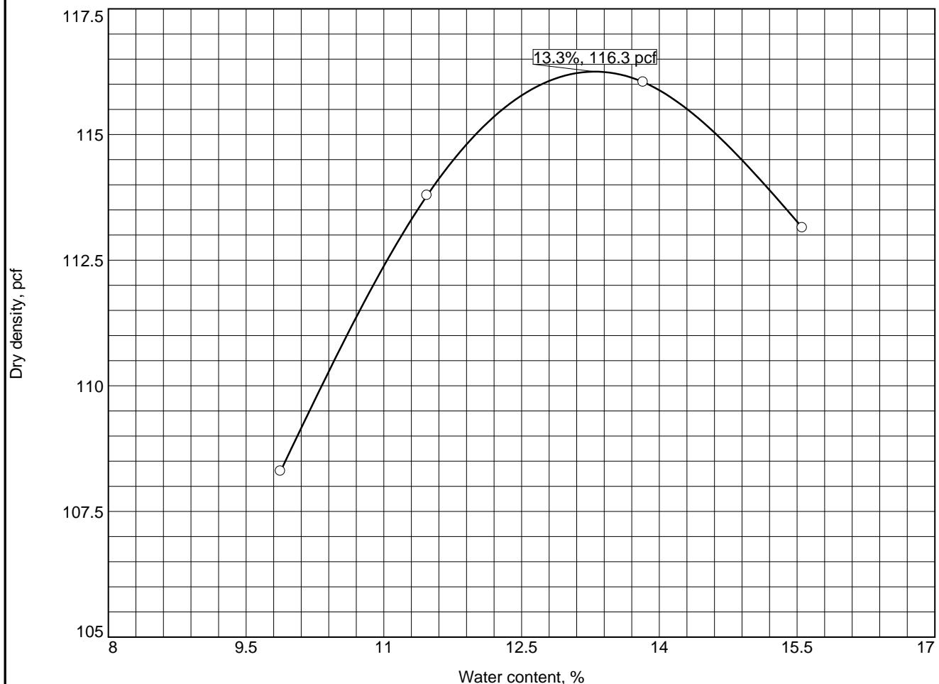
Test specification: ASTM D 698-07 Method B Standard
